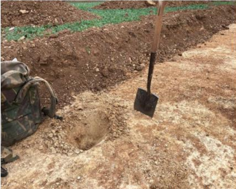
Above, Limestone is 'weathered' / 'altered' rather than solid. Few very fine roots, but very dense and compact so probably only rootable for about 20cm.
